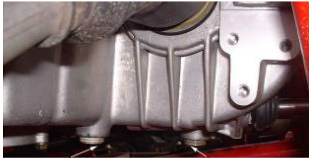
outlet of iron dust oil transmission outlet
